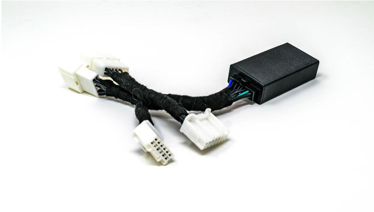
Before proceeding installation select desired behavior using the switch on the backside of the controller. Slider switched to the right will lower the windows, after the convertible top is open. Slider switched to the left will raise windows after the convertible top is locked in the open position.
